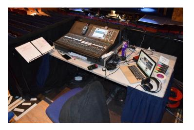
A member of staff operates the **sound desk**. This controls the sound of the actors' microphones. Only the sound operator can touch this.
